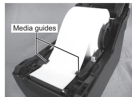
Printed side should face upwards
