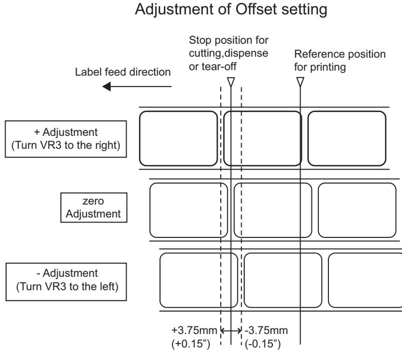
In addition to the above setting, the Offset position can also be adjusted by using SATO Utilities Tool application or by sending command <PO> from the host. The setting range is within  $\pm 99$  dots. (One exception is for the Tear off mode; for the Tear off mode, the range is -60 dots to +99 dots). This setting is normally not necessary. Use **VR3** potentiometer on the printer for permanent setting.
