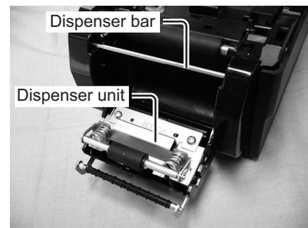
3. Peel off the first two leading labels from the liner (backing paper) and then load the label roll on the **media holder**. After pulling out the leading liner (backing paper), pass the liner (backing paper) through the **media guides** and then pass over the **dispenser bar** so as to cover it. Then pass the liner (backing paper) under the **pressure bracket** as shown.
