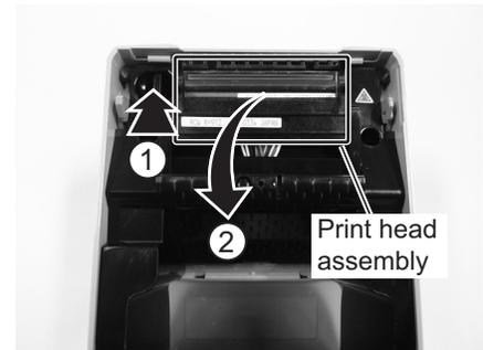
4. The **cable connector** (circled) at the rear of the **print head** is now exposed. Pull the print head downward, then gently disconnect the **print head** from the cable connector.
