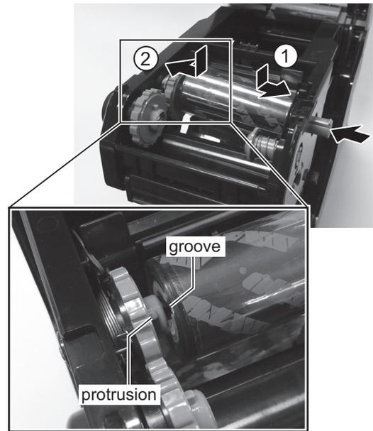
4. In Mount the empty ribbon core on the **ribbon wind-up unit** the same manner as in step 3 above.
