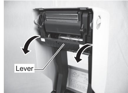
4. On the right side of the **ribbon unit**, press the catches at both top and bottom to remove the **side cover**. Move the whole **print head assembly** downward.
