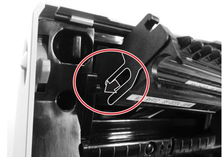
7. Press and hold down the **side tab** (see arrow ①) which was previously used to release the **print head**. Push the **print head** upwards so that it snaps into place.
