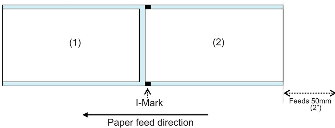
The printer behavior paper end is detected is as follows:
