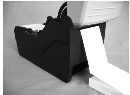
3. While holding the **media guide slide lever**, adjust the width of the **media holder** ① to match the media size. After pulling out the media, pass the media through the **media guides** and place the leading edge of the media on top of the **platen roller**.
