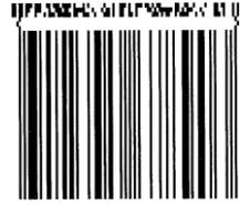
[Coding example 9] EAN-8 Composite(CC-A/CC-B)
