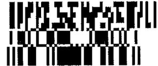
[Coding example 4] DataBar Stacked Omni-Directional Composite(CC-A/CC-B)
