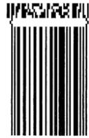
[Coding example 8] EAN-13 Composite(CC-A/CC-B)
