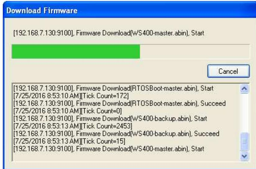
9. When the data transmission is complete, your printer starts to update its firmware. During the update, LED 2 turns to red and orange alternatively, while LED 1 turns to solid green. In the **Download Firmware** dialog box, the message shows that your printer is updating the firmware.
