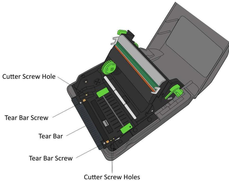
4. Remove the tear bar from the printer.
