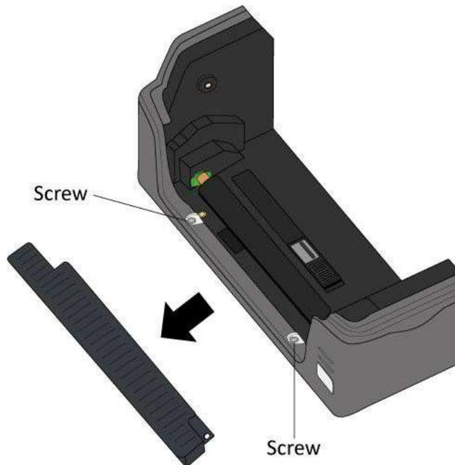
6. Loosen and remove the two screws on each side of the **Media Roll Holders**.
