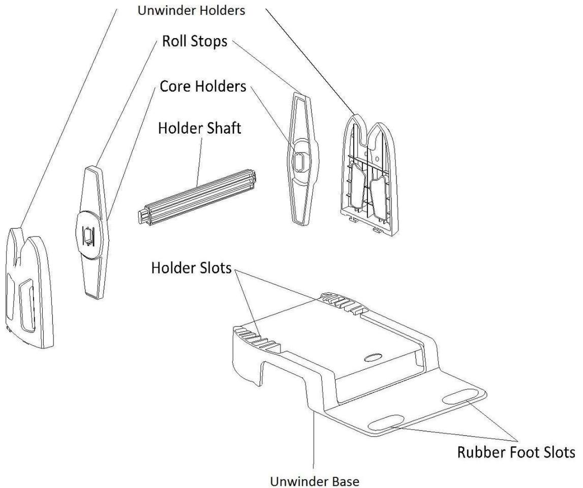
To install an external unwinder:
