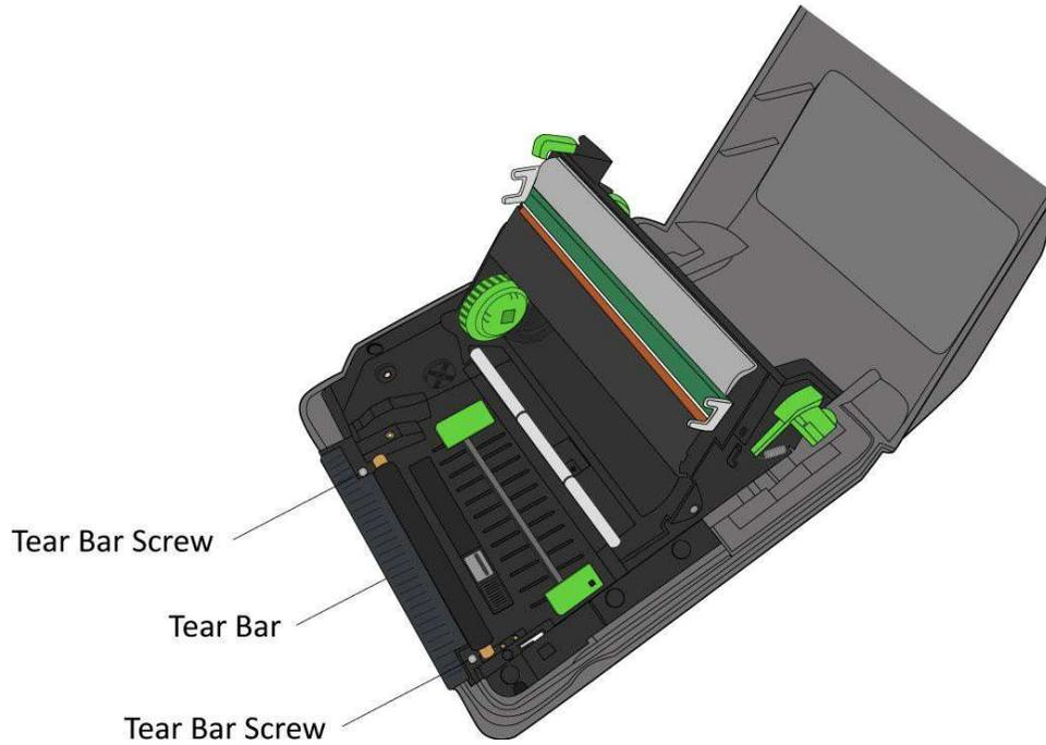
4. Remove the tear bar from the printer.
