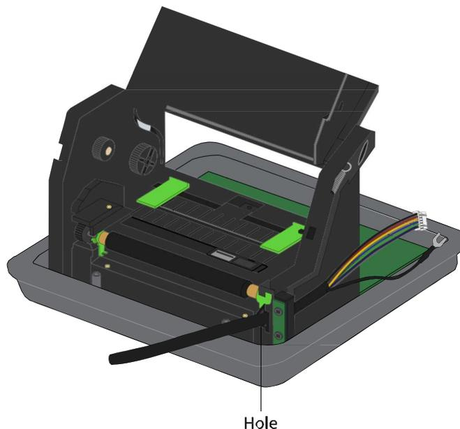
2. Plug the cutter connector to the **J8** on the main board. **J8** is a white port
