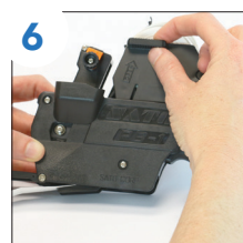
After securing the roll of labels onto the spindle and placing the guide on top of the roll of labels, close the label roll door.
