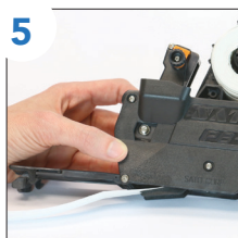
Drop the labels down the center of the tool, gently feeding the end through until it slides out the bottom.
