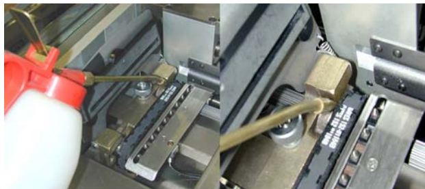
PLACE 2 DROPS OF OIL ON SHAFT AT THIS LOCATION
