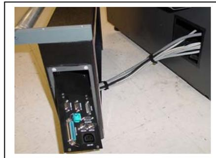
7. Remove the filler plate from the Web Guide Box and discard, retain (4) 6mm screws.
