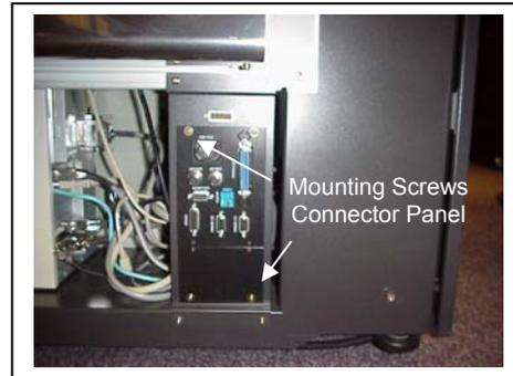
3. Remove the four mounting screws securing the connector panel to the mounting bracket.
