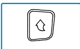
This button is used to feed the paper manually or return to the previous step.
