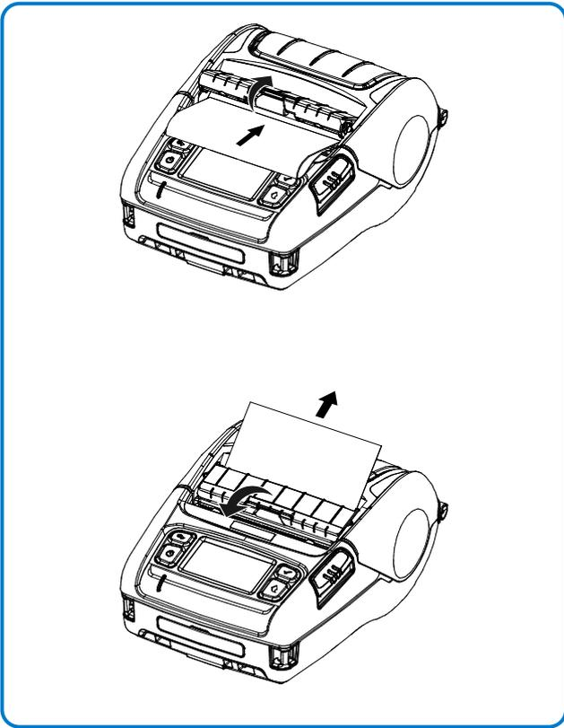
1) Insert the paper after open the peeler as shown.
