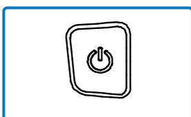
This button is used to turn the printer on, off, to move to main menu or to operate the action.
