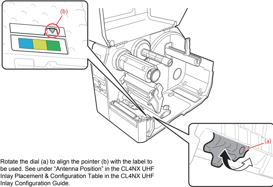
Rotate the dial (a) to align the pointer (b) with the label to be used. See under “Antenna Position” in the CL4NX UHF Inlay Placement & Configuration Table in the CL4NX UHF Inlay Configuration Guide.
